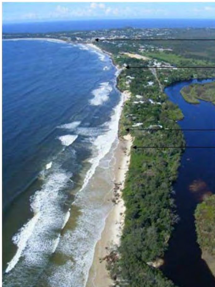
Belongil Beach after May 2009 storm (from Helman 2010), note the lack of a beach in front of walls and accelerated erosion of the spit at the end of the wall.
